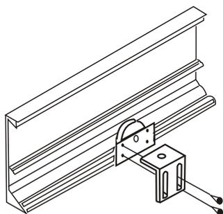
2 According to the length of faceplate, fix the two fixing lugs on the side of the tracks
